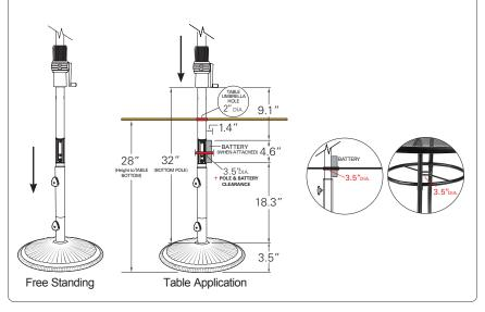
Attach rechargeable battery pack onto bottom pole.
