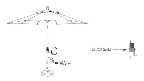
To tilt, simply twist the collar in clockwise direction.
