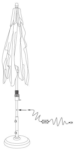
**Note:** The transformer output power is 12V. It is normal for transformer to get warm after long period of use. Avoid sun on power supply/transformer to increase lifetime use. Be sure not to drop transformer. *Note: Use only the Power Cord/Transformer supplied.*
