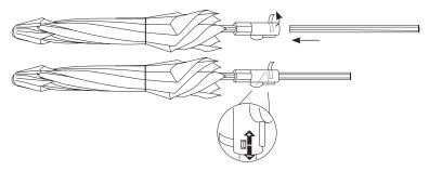
· Close release clamp to lock bottom pole into canopy/mainframe.
