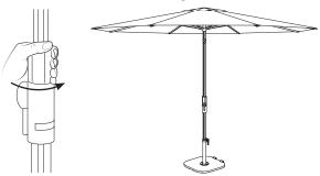
• Gently pull down handle and lift up to engage crank.
